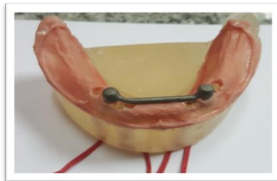
Figure 9. Strain gauge orientation on the mandibular cast with bar attachment
