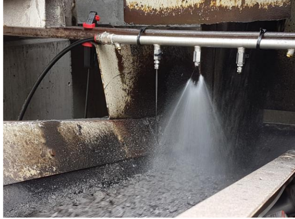
Figure 9: Rejuvenator addition to RA on the conveyor belt utilizing a spraying system [34].
